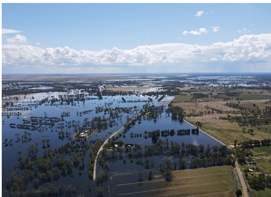
Left: Murrabit West Road (centre left) looking West, showing homes surrounded by water and Goulburn-Murray Water channel acting as levee bank preventing further flooding (photo courtesy Paul Oswin).
