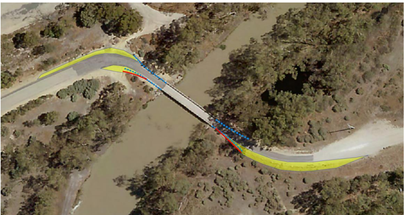
Figure 3: Pratt Rd Bridge – Proposed Approach Improvements.
