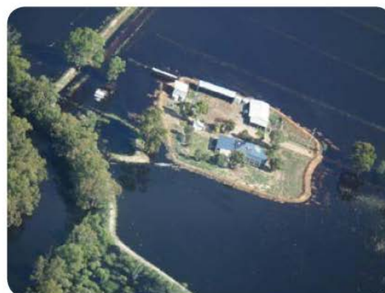
Temporary levee around property in Benjeroop, 2011 flood
